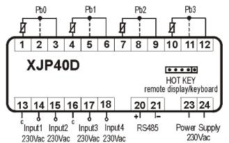
Pt100 2 wires: connect to not dashed terminal 24/110Vac Power Supply: connect to 23-24 terminals
